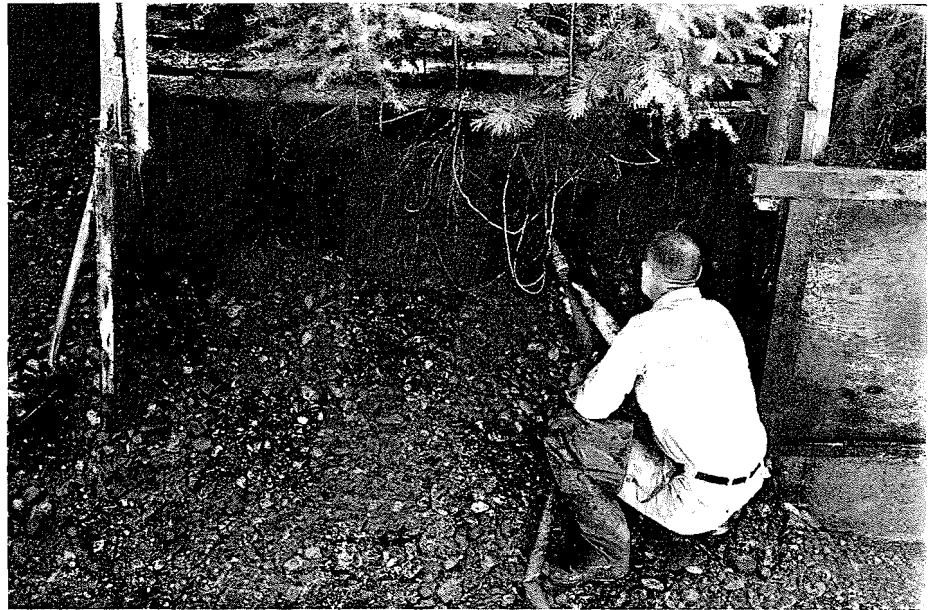
FIG. 2. Root washing and extraction in a rock bin. Soil was washed from the roots by water under low pressure. Trees were removed from the cross supports as their roots were extracted from the soil and rock mass.
