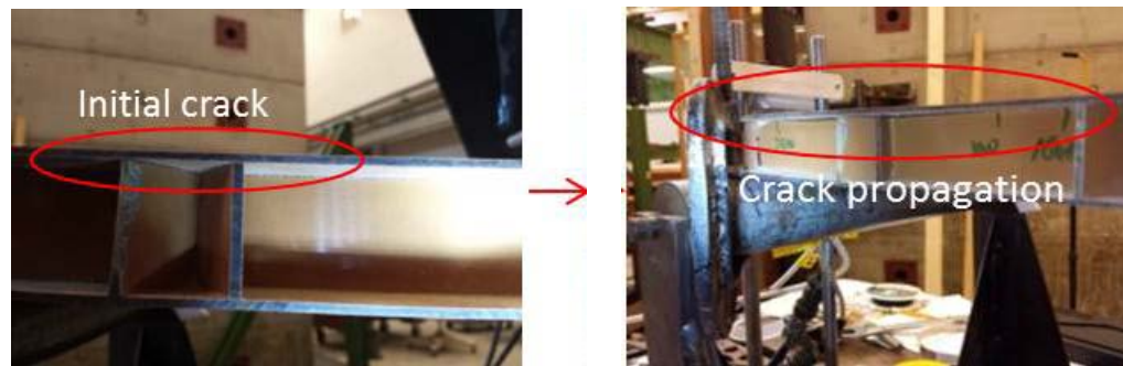
Figure 10. Damage propagation under cycle loading in imperfect sandwich beam.
