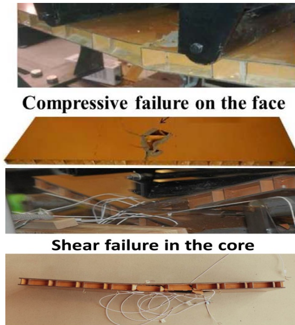
(a) Face failure
