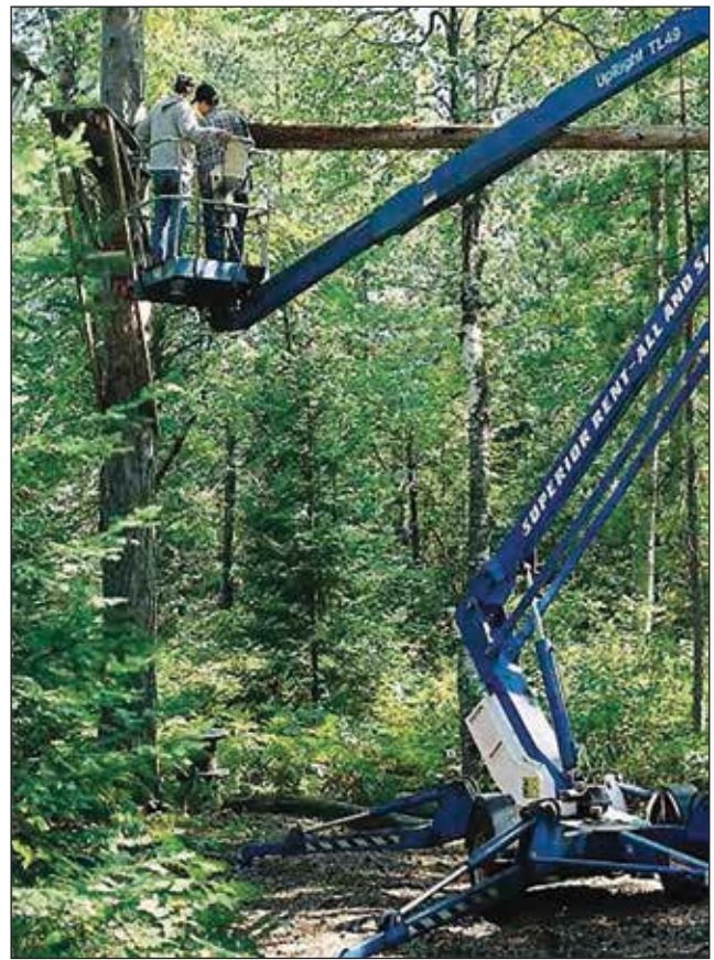
Figure 7.8—Case study at the U.S. Forest Service Nesbit Lake Camp, Sidnaw, Michigan—Visual and nondestructive evaluation of red pines supporting a ropes course.
