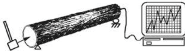
Figure 8.4—Resonance acoustic measurement on a log.
