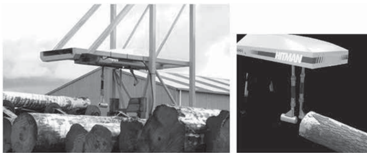
Figure 8.17—Hitman LG640 automated log grader installed on the debarker out-feed. (Photo on the right shows the swinging hammer and microphone sensor.) (Photo courtesy of Fibre-gen Ltd.)
