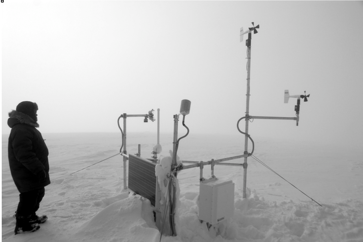
Figure 12. Ilkoo Angutikjuak examines the Akuliaqattak Station (70°18'50"N, 68°9'24"W) in near whiteout conditions. Note temperature/relative humidity sensor on center leg, which has been bent by a visiting polar bear. Two such bear incidents have fortunately not compromised measurements.
