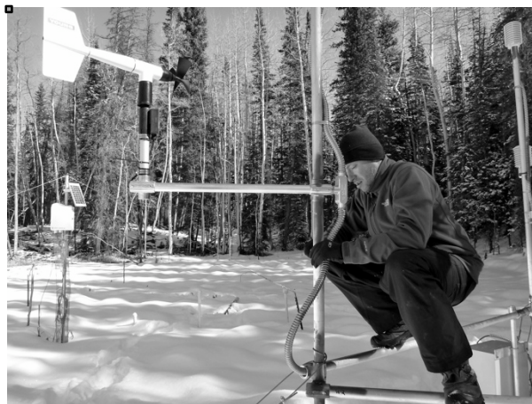
Figure 11. Daniel Bowker tightens hose clamps above and below a cross arm to secure flexible conduit. Wires were combined in all possible runs to reduce the number of individual conduits and connectors, as well as the number of ports into logger and battery boxes.
