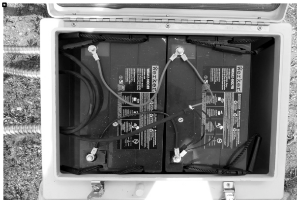
Figure 8. Battery box configuration. The two conduits at the upper left location come from the two solar panels. The lower conduit has solar and 12 V power from the batteries all going to the solar controller in logger enclosure.
