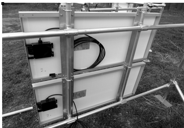
Figure 9. Dual 70 W solar panels mounted on tower cross arms. We have used Nu-Rails, U-bolts and aluminum plates to mount the panels, but many different configurations can easily be used for mounting.
