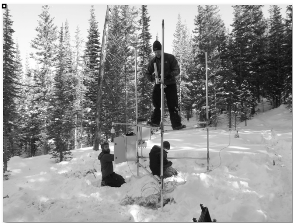
Figure 17. Daniel Bowker hangs the lower anemometer while Roger Tyler and AJ Marsh wire instruments and data loggers at a wetland location at the Fraser Experimental Forest.
