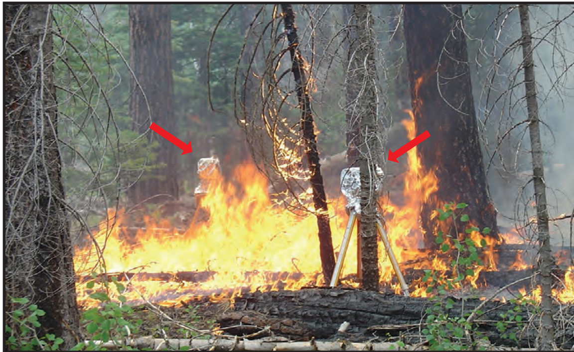
Fire-behavior packages mounted on tripods gathers data for energy transport modeling as a wildland fire burns around them
