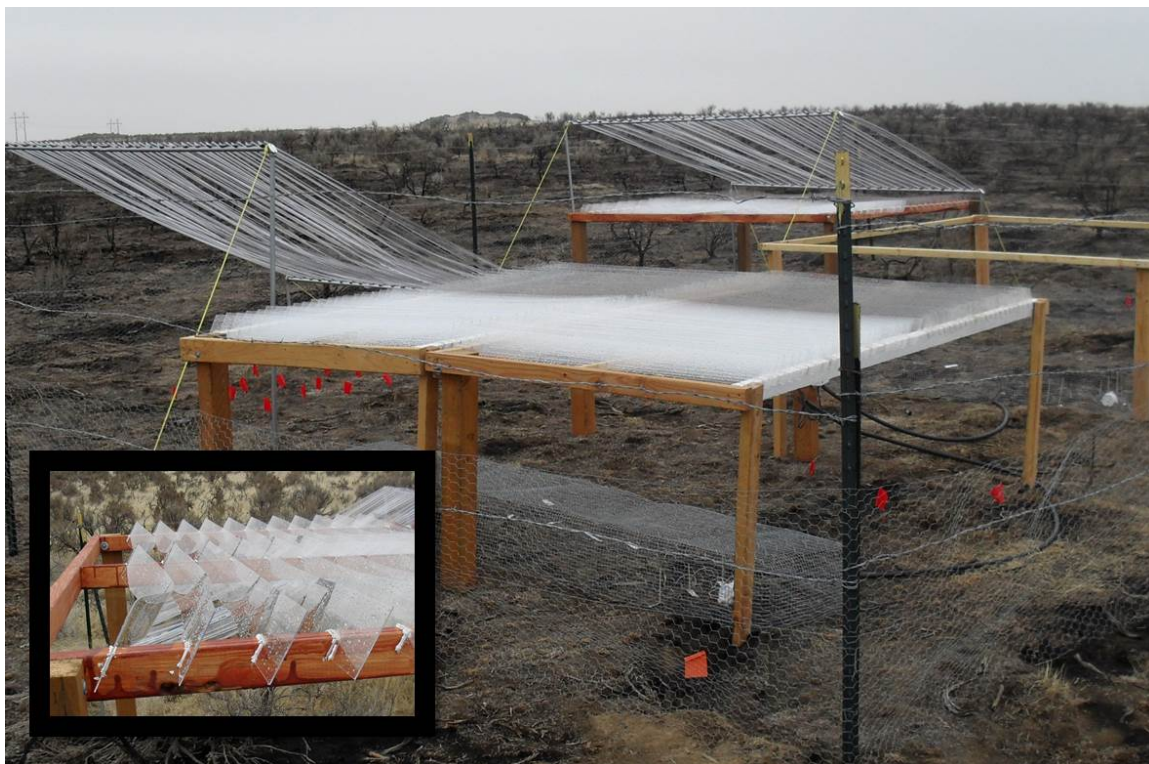
Figure 9. Photo showing style of warming and control chambers. In photo, the leftmost chamber is the warming device, and two chambers having rainout shelters in the back row are rainout treatments for a related project. Inset picture shows cross section of roof design.
