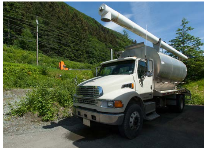
The Sealaska Building in downtown Juneau (upper right) is heated in large part by this fully automatic 750,000 Btu/hr KÖB/Viessmann pellet boiler (above). Wood pellets are delivered several times a month in bulk by this converted grain delivery truck (right).
