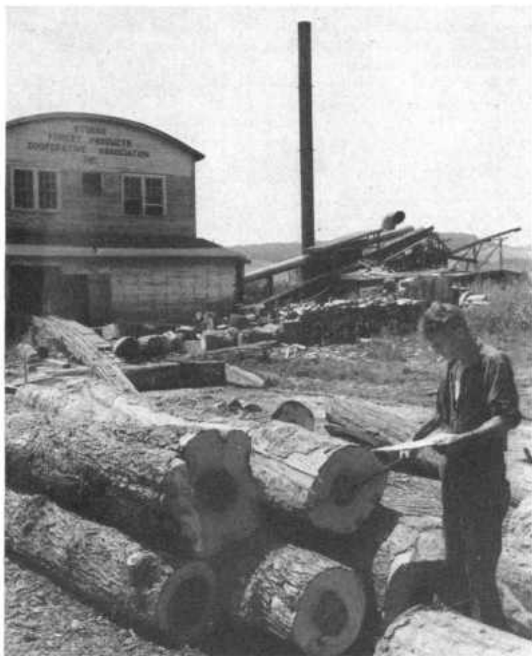
FIGURE 5.—All logs are scaled and graded at the sawmill. This careful attention to quality assures members a fair price for their logs.
