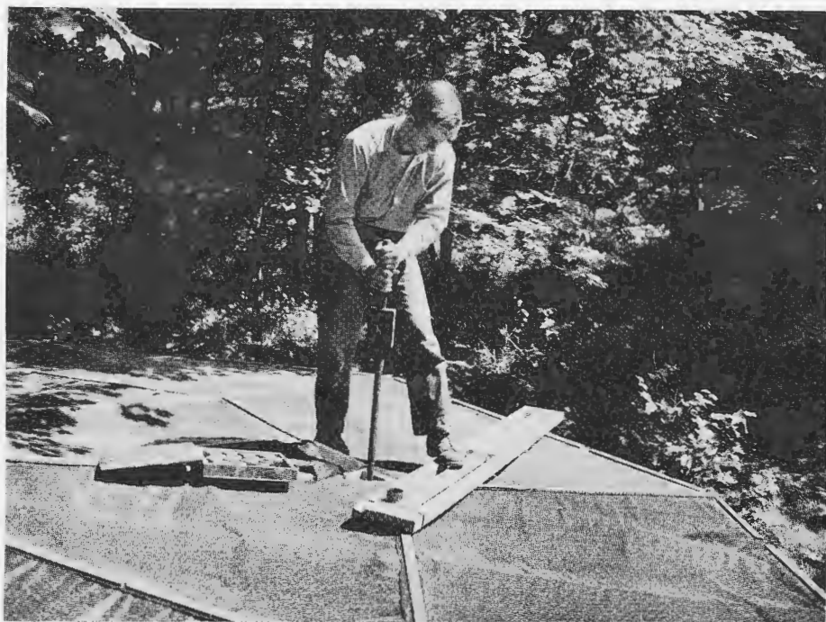
Part V, Fig. 7. Soil moisture measurements were taken through trapdoors in the intercept platforms.
