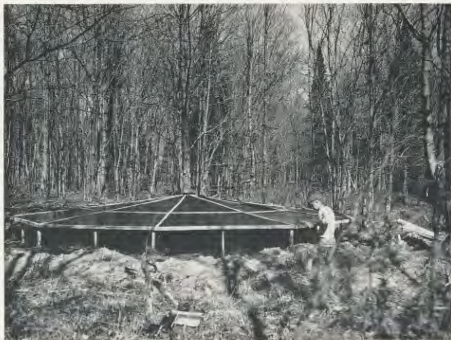
Below: Part V, Fig. 5. Moisture-intercept platform for 100 % moisture reduction.
