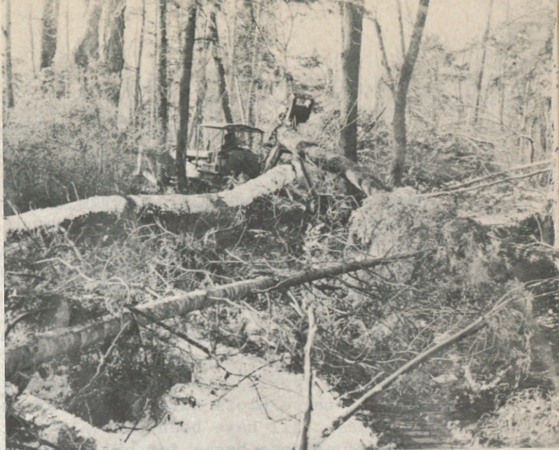
Figure 1.--An HD-5 tractor skidding tree-length "stringers" with a Carco-type arch during a partial cutting operation in Marquette County, Mich. Since a capital investment in young growing stock remains on the land, logging damage to the residual stand must be held to a minimum.
