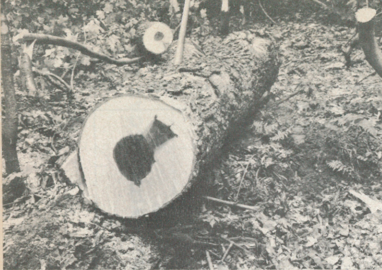
Figure 8.-- Upper Photo : Fan-shaped discolorations beneath small, callused-over scars extend only toward the heartwood. These dark, brown stains are arrested from progressing outward into the bright callus wood. This is the usual pattern of this defect except in scars infected by sapwood-rotting fungi.
