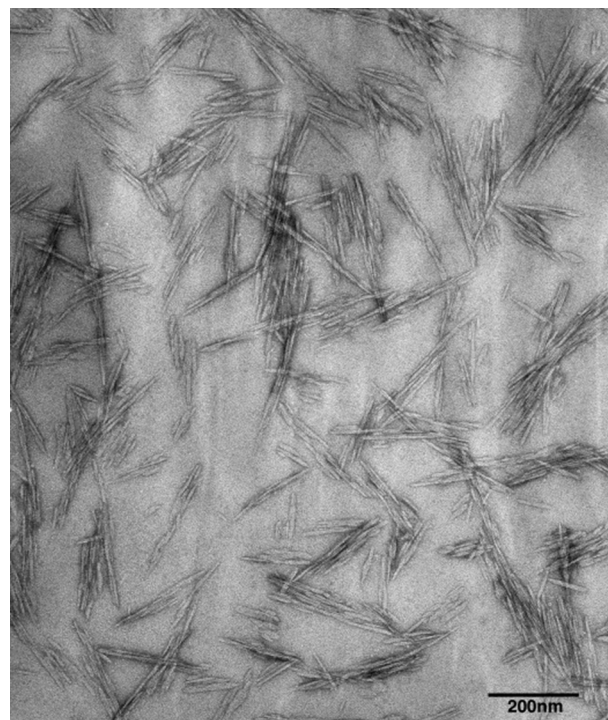
Fig. 1. TEM image of wood-derived CNCs.
