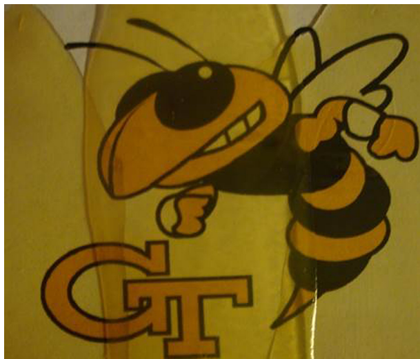
Fig. 4. Photographic image of epoxy/CNC films. From left to right: 5, 2, 0 wt.% CNC.
