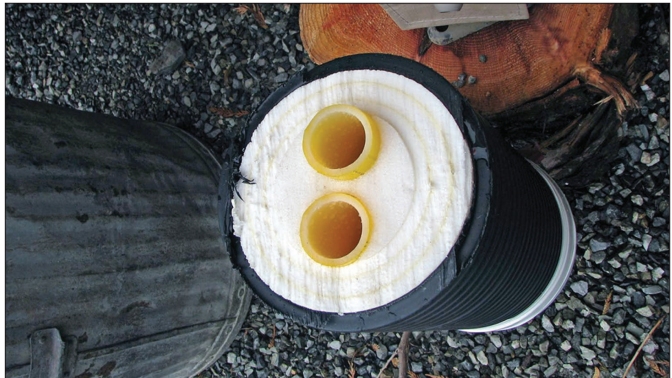
Figure 2—Cross section of insulated piping for water distribution, showing layered construction and supply and return pipes, normally buried underground.
