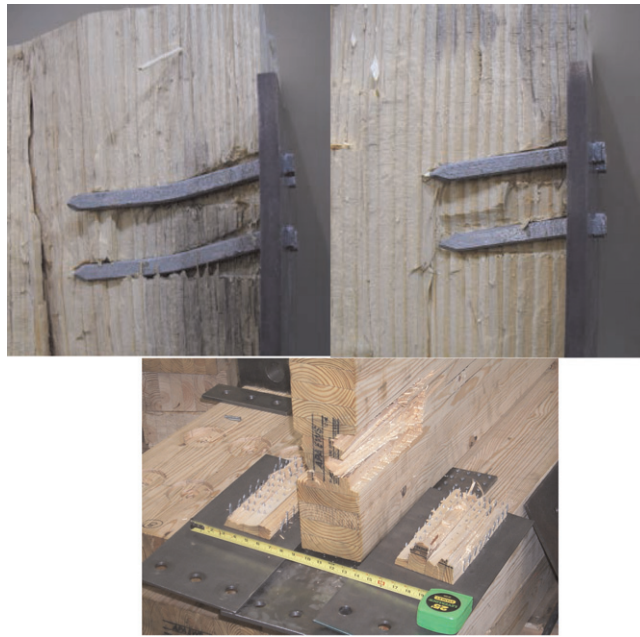
Figure 7 Timber rivet failure modes: (clockwise from top left) rivet bending, rivet bearing, and wood tear out.
