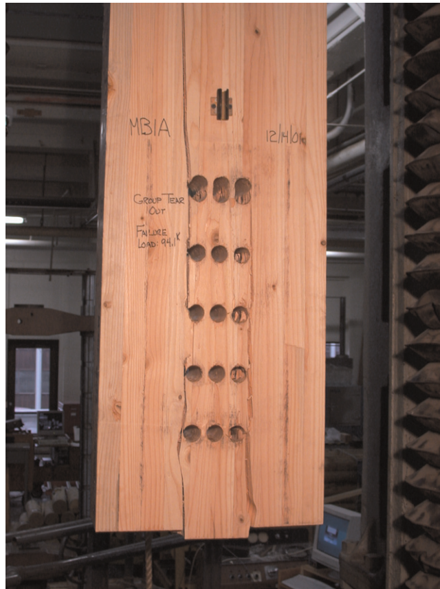
Figure 6 Failure of the multiple fastener connection due to group tear out.
