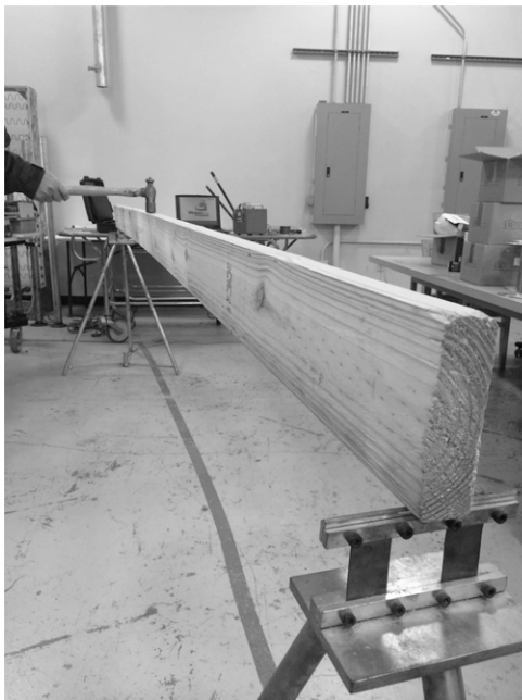
Figure 2. Transverse vibration evaluation: E-computer Model 340.
