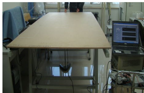
Fig. 2. Vibration testing apparatus for assessing the mechanical performance of full-size wood composite panels. (a) Schematic of vibration testing under free-free support condition. (b) Laboratory vibration testing of a full size panel.
