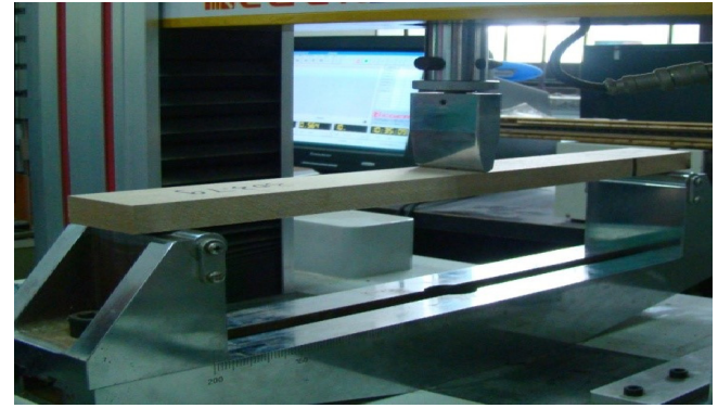
Fig. 3. Flatwise static bending test on a small specimen cut from the wood composite panels.
