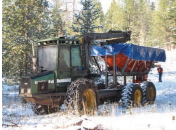
A forest site being treated with pellets using a custom biochar pellet spreader mounted on a forwarder. Photo: Nate Anderson
