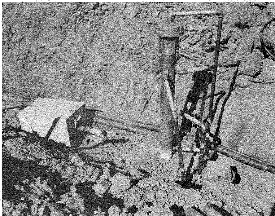
Figure 2.--Simulated air intake vent installation showing protective piping for leading off thermocouple wires.
