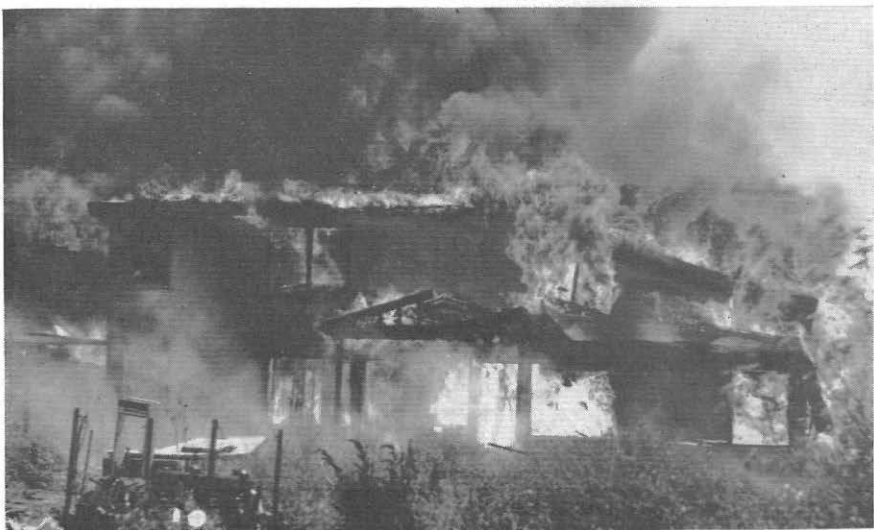
Figure 1. View of first Richmond test fire 33 minutes after ignition (described on page 5).
