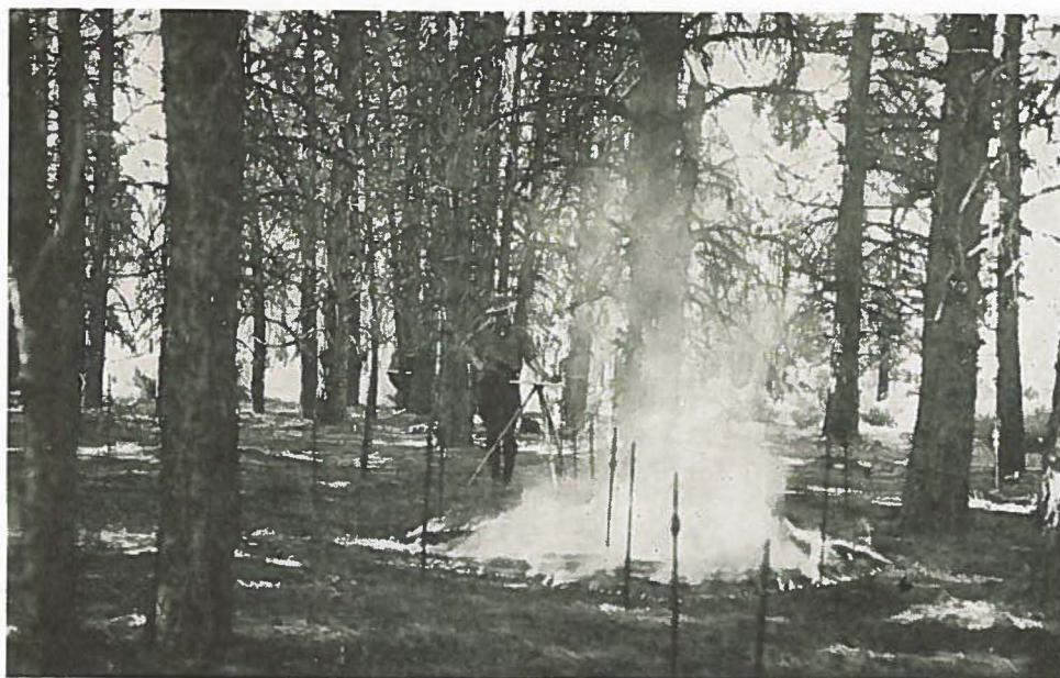
FIG. 2 TEST FIRE IN EVEN-AGED STAND OF PONDEROSA PINE; 8 MIN AFTER IGNITION
