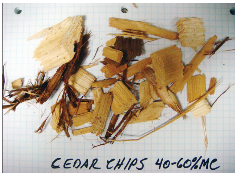
Figure 14—Cedar chips from fuel bin with moisture content of 40 to 60 percent.
