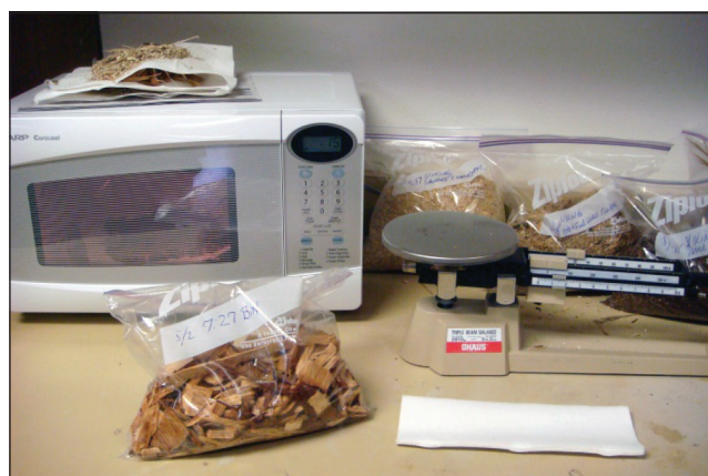
Figure 15—Equipment for determining moisture content using ASTM E1358 (microwave method).
