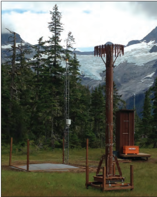
One of two new weather monitoring stations in Héén Latinee Experimental Forest. The data will be used for research and by the National Weather Service to improve weather forecasting.
