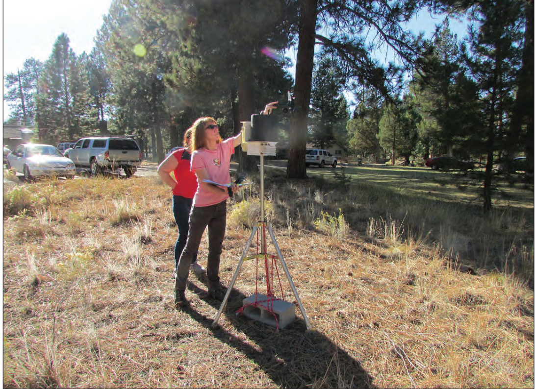
Scientists set up a meteorological monitor prior to a prescribed fire in the Deschutes National Forest. The data from this and 12 other monitors were used to model smoke movement and intrusion into Bend, Oregon.
