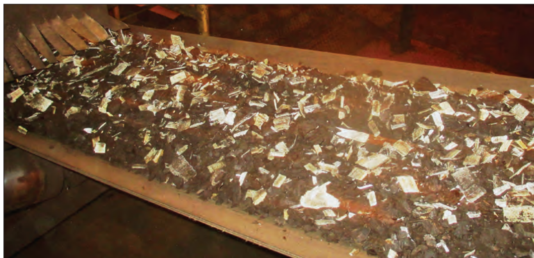
A wood-coal cofiring test burn at Aurora Power in Fairbanks, Alaska.
