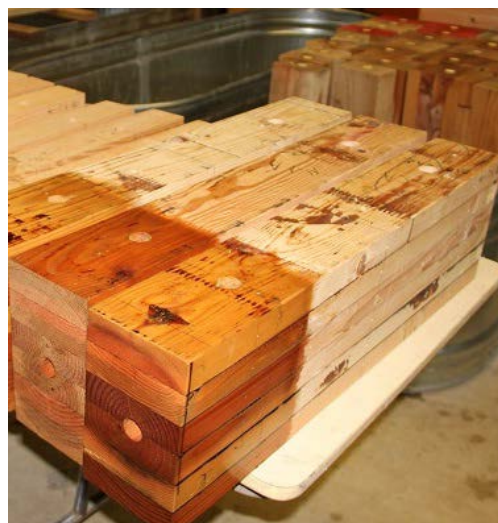
Figure 2. Fungal cavity holes in specimens. a) Locations of the drilled holes. Units shown are inches. b) Image of the holes drilled in a six-laminate glulam.
