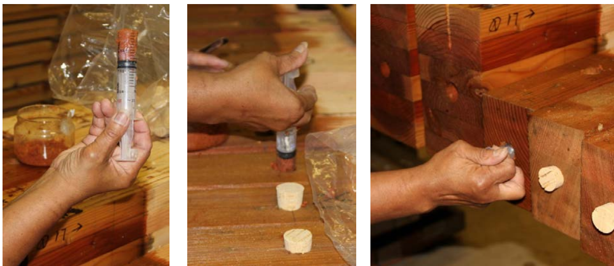
Figure 5. Inoculating specimens with Fomitopsis pinicola , brown rot.
