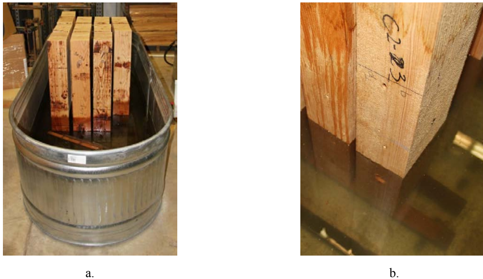
Figure 4. Pre-soaking specimen prior to inoculation. a) Specimen placement in the soaking tanks. b) Water level at least 2 in. (51 mm) above drilled holes.
