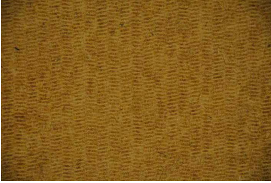
Figure 1 Uncoated cellulosic fiberboard (top view).
