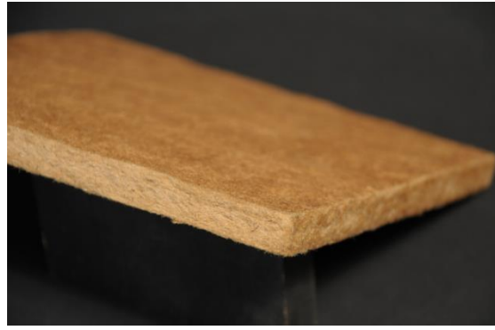
Figure 2 Uncoated cellulosic fiberboard (side view).
