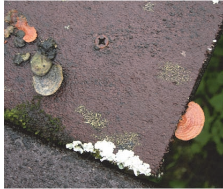
Figure 1: WPC in field exposure in Hilo, HI with wood decay fungus fruiting body after 2-3 years.
