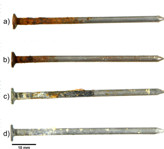
Fig. 4. Images of the fasteners after being removed from the 1-year field exposure test. (a) steel fastener in treated wood, (b) steel fastener in untreated wood, (c) galvanized fastener in treated wood, (d) galvanized fastener in untreated wood.
