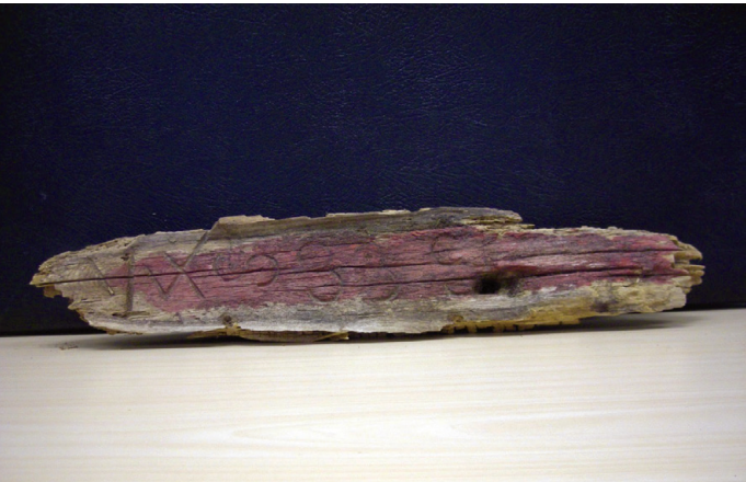
Figure 2. —A longitudinal section of an original bearing-tree scribe housed at the Superior National Forest Supervisor’s Office. Note how the corner location information was scribed vertically on the tree bole due to small diameter size. Approximate size of wood section is 61 cm (24 inches) long by 10 cm (4 inches) high by 4 cm (1.5 inches) wide. Photo by Casey McQuiston, U.S. Forest Service.
