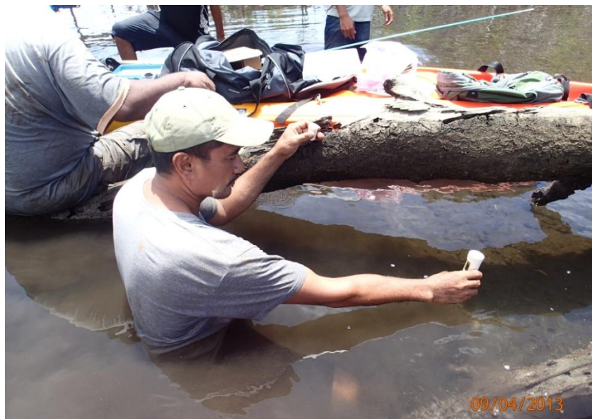
Figure 5. Seawater salinity, pH, and temperature were all measured with this device. In all cases, the probe of the sensor was positioned at 1 inch (2.54 cm) below the water line.
