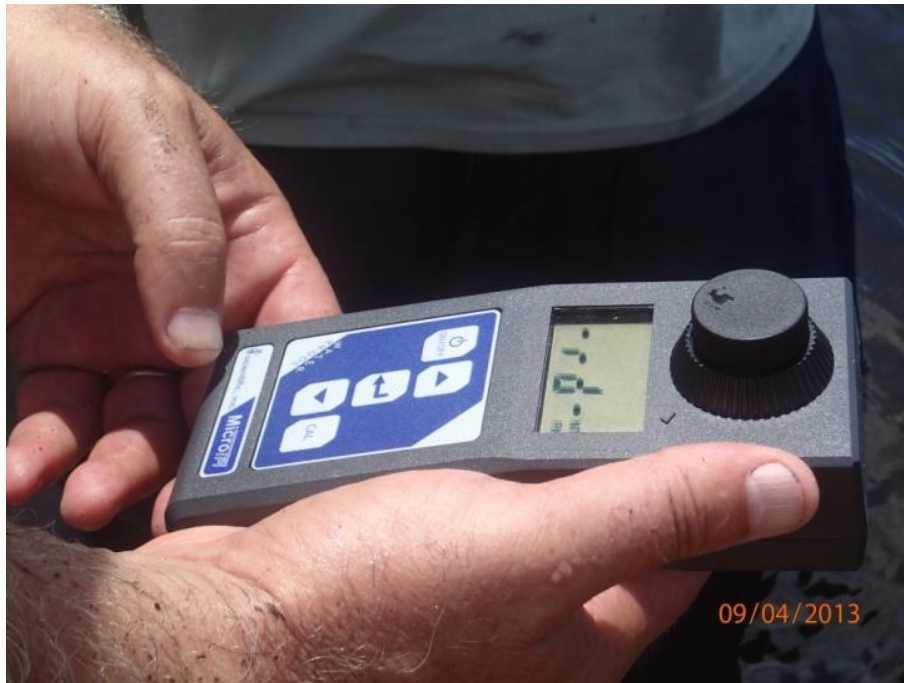
Figure 4. The use of a turbidity meter is straightforward, although calibration of this instrument is more involved. Water samples are collected in a cuvette (a 3-cm-long glass vial with a plastic, screw-on top, shown at the right in the photo above) and then inserted in the meter. (Photo by M. Falanruw).
