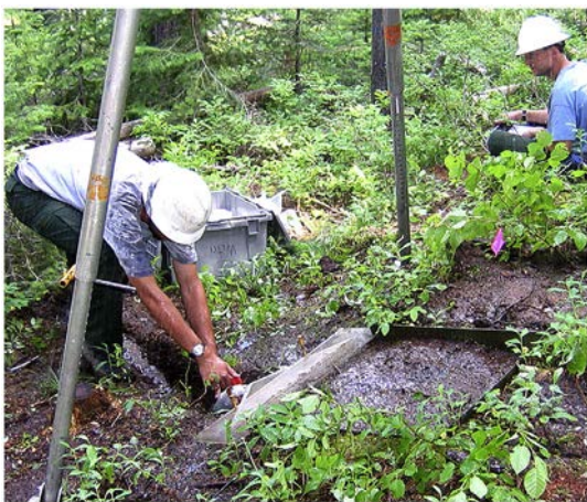
Fig. 2. PF5 rainfall simulation on a bare plot in an unburned site. The surface vegetation, litter, and duff were removed from the plot and the area immediately adjacent to the plot. (Photo credit: USDA-Forest Service J. Yost).
