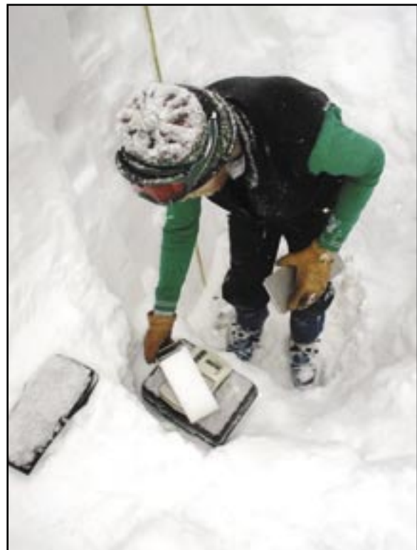
As part of the Cold Land Processes Experiment, snow density measurements are taken to get total snowpack water equivalent
