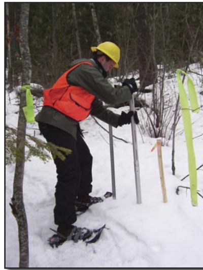
A Station researcher measures the snow water equivalent as part of a fuel management study in the Priest River Experimental Forest, Idaho.
