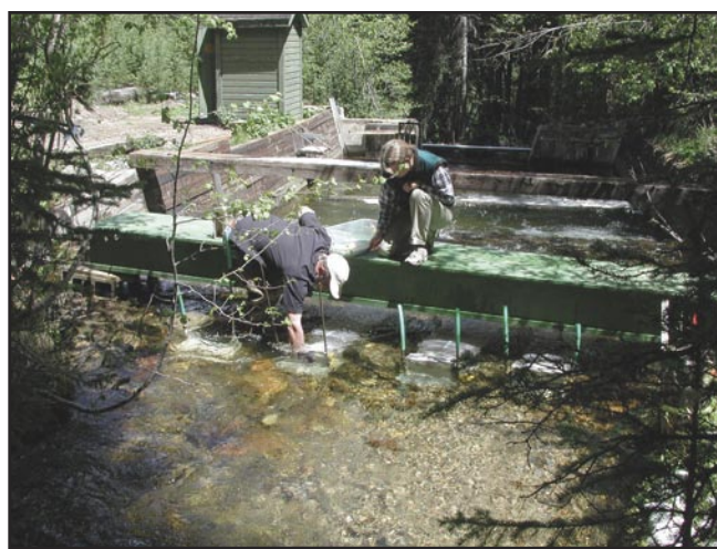
Researchers empty a portable bedload trap at the Fraser Experimental Forest in Colorado.
