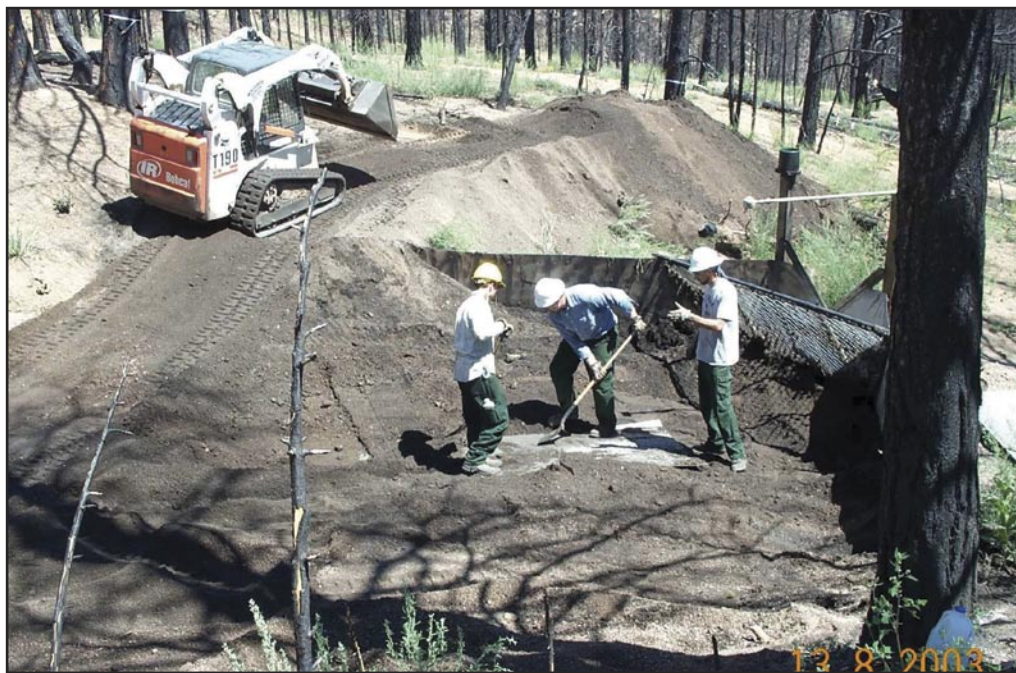
Researchers clean out sediment deposited by a single storm runoff event from a high severity burned area on the Hayman Fire, Colorado, September 2003.
