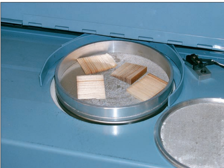
Figure 5—Dead fuels (excelsior, 3/4-inch dowel, 3-inch slice) used in the evaluation of quick-response ovens in test 1 and test 2. (Photo courtesy of USDA Forest Service)
