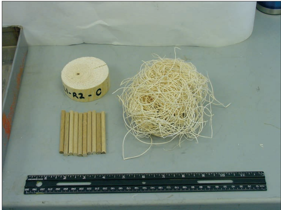
Figure 2—Fuel types used in container evaluation study. The fuels are (clockwise from right) aspen excelsior, 1/4-inch diameter pine dowel, 3-inch diameter lodgepole pine post.
