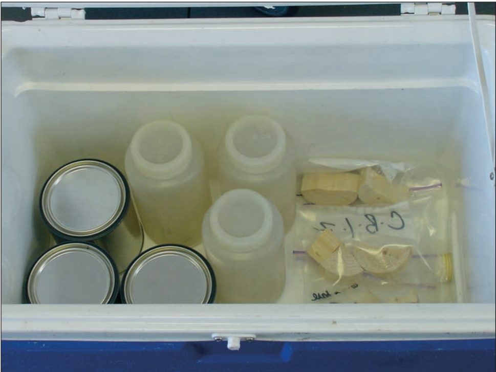
Figure 1—Three types of containers used in fuel storage container study. The containers are (from left to right) 1-quart steel paint can, 32-ounce autoclavable polypropylene bottle, and 1-quart self-sealing freezer-grade polyethylene plastic bag.
