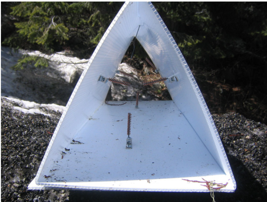
A DNA-collecting device that works well for fishers is an open-ended triangular box that collects the animal's hair using side-mounted metal gun brushes (photo by Michael Schwartz, USDA Forest Service).
