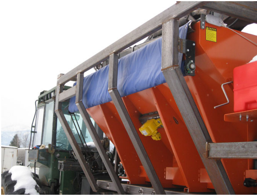
Figure 4 —Custom rain tarpaulin system that can be actuated from ground level (photo by U.S. Forest Service).
