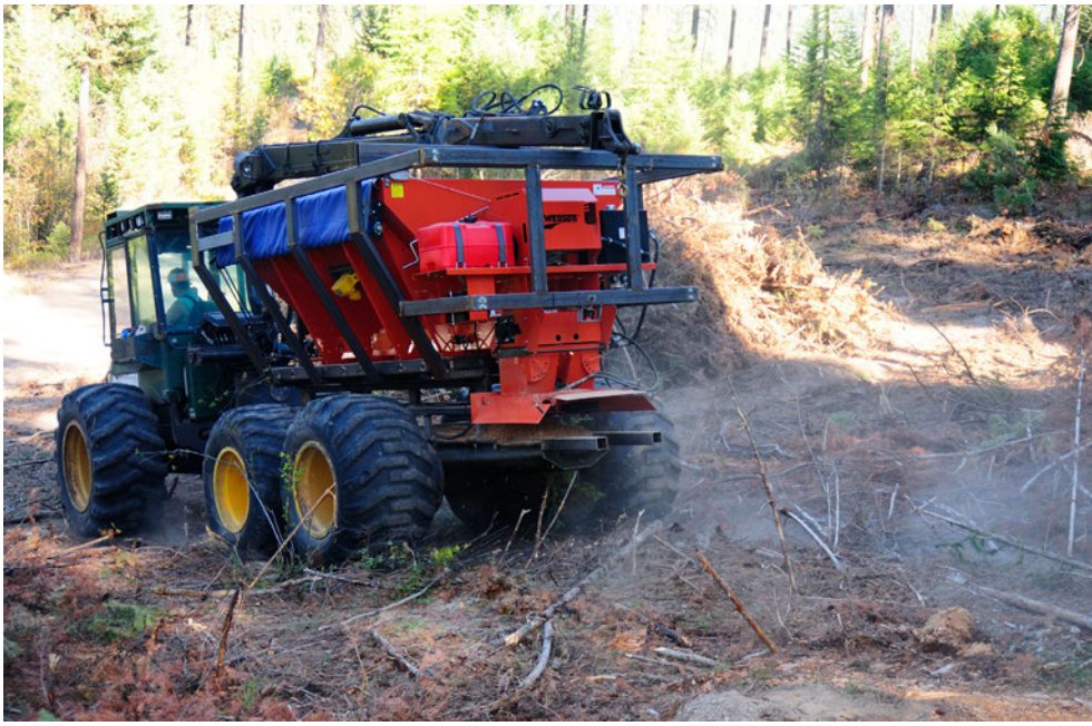
Figure 1 —Forwarder with prototype biochar spreader within a protective cage on test site, Ninemile Ranger District, Lolo National Forest, Montana (photo by U.S. Forest Service).
