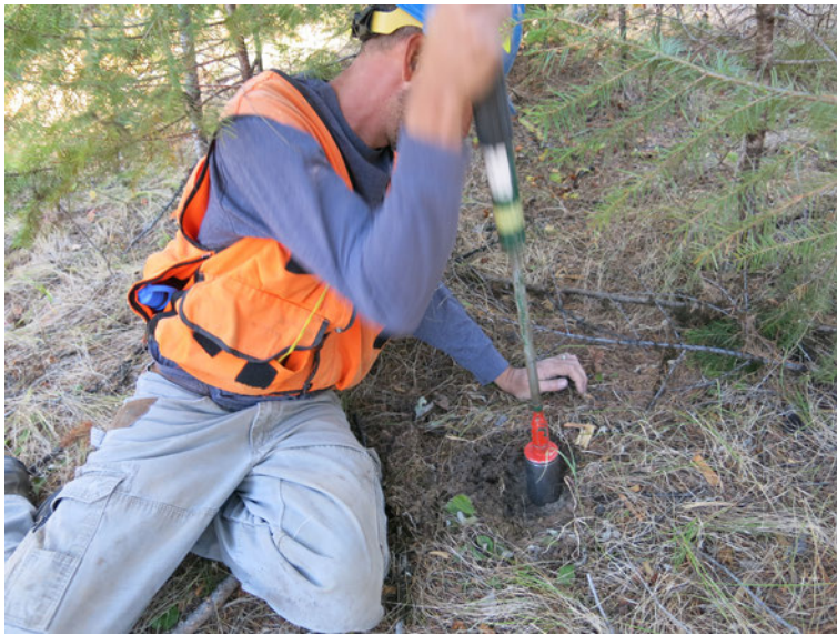
Figure 7 —Soil scientist using a slide hammer corer to collect samples for measurement of soil compaction (photo by U.S. Forest Service).
