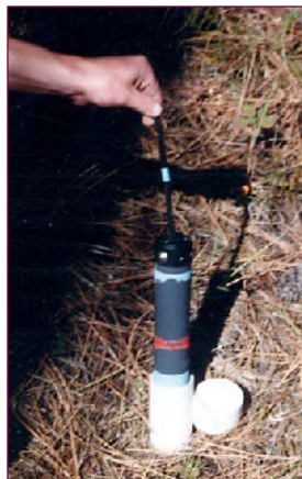
Inserting probe in a PVC pipe enables correct measurement.
