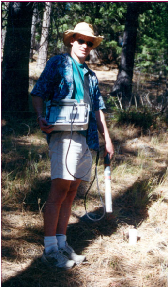
Greg Peters with a Sentry 200 Troxler used to measure volumetric percent soil water content.
