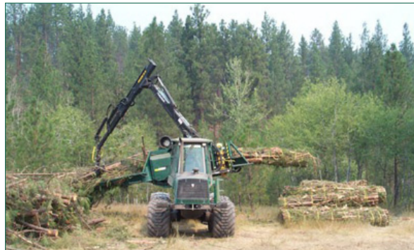
A slash bundler collects biomass as part of a field trial in the Bitterroot Valley to study the economics of collecting and using biomass from fuel reduction projects compared to burning it on site. (Photo courtesy of the USDA Forest Service.)
