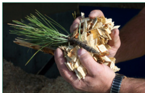
Biomass boilers use wood chips, needles, and bark from hazardous fuel reduction projects to provide efficient fuel for school heating systems and reduce air quality impacts from open burning of wood materials. (Photo courtesy of USDA Forest Service.)
