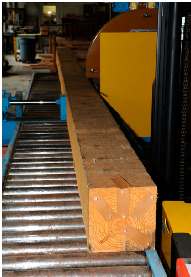
Figure 1. Southern pine beam as delivered to Forest Products Laboratory. The cardboard pinned to the end grain shows the orientation of samples cut along the true radial direction.
