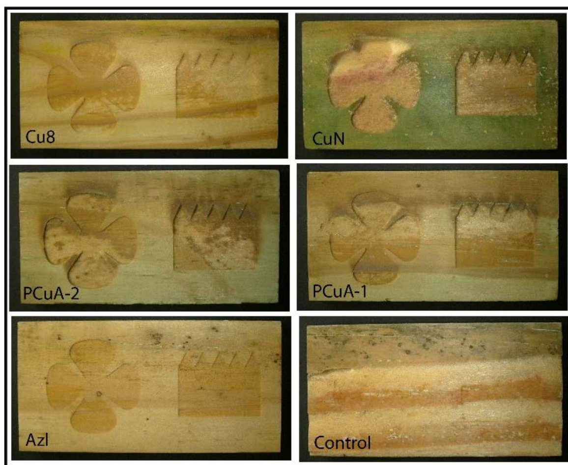
Figure 5: Specimens showing preferential feeding within laser-marked areas on solid pine test blocks (note: little feeding on blocks treated with Azl; laser markings on untreated, control specimens are no longer visible)
