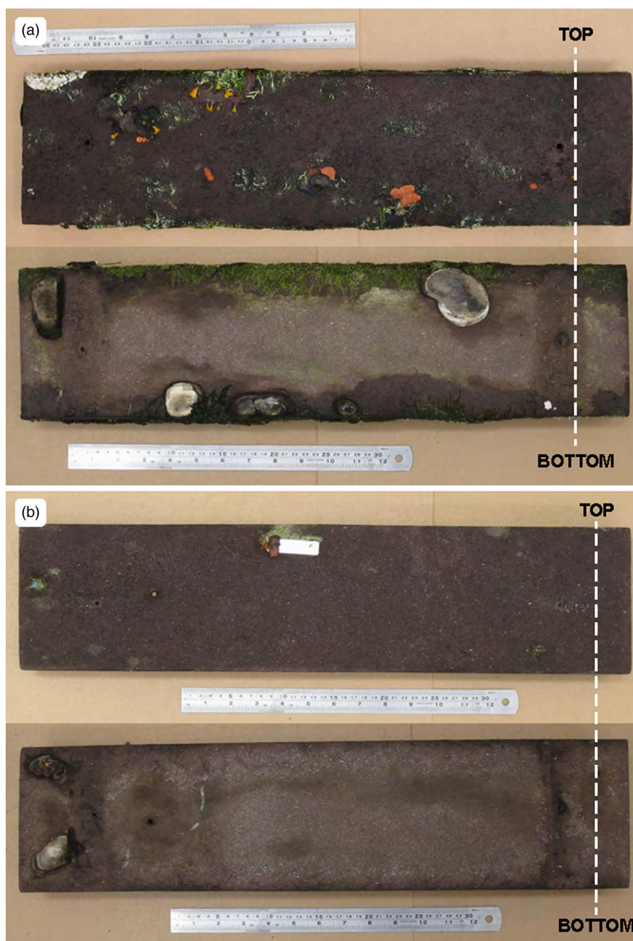
Figure 3. Top and bottom views of the (a) Shadow board and (b) Sun board obtained from the field after 8 years of exposure; the dotted line indicates the vicinity of where samples were taken for density measurements and CT imaging.
