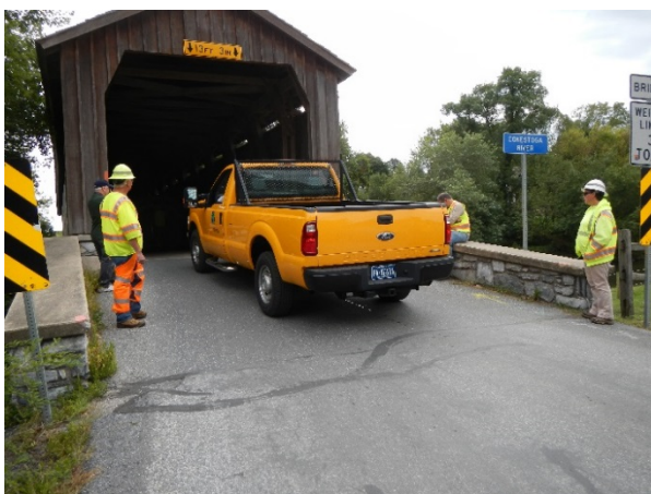
Figure 17: Pennsylvania Dept. of Transportation light truck loading of Hunsecker Bridge
