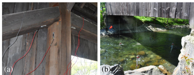
Fig. 4. Representative live-load-response measurement instrumentation setup: (a) member strains; (b) global deflections (images by Travis K. Hosteng)
