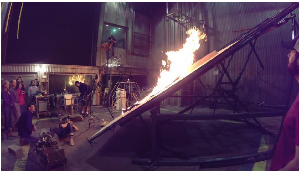
Photo: Researchers are preparing for the next phase in examining physical fire processes by adding the effect of slope and fire-on-fire interaction. The apparatus in the photo above can be set on an angle as shown as well as in a V-shape to begin to simulate fires in complex terrain. Photo courtesy of Mark Finney / FFS.
