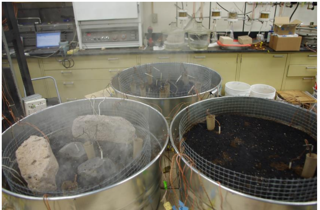
Top photo: The flaming front approaches masonry in an ArcBurn flame test. Bottom photo: Smoldering tests are performed on all artifact types (masonry, ceramics, chert, and obsidian). The masonry (tan) and obsidian (dark gray) can be clearly seen in the test bed. Photos by Rebekah Kneifel.
