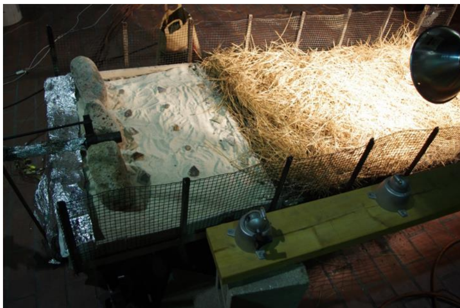
Photo: This photo shows the pre-burn setup of ArcBurn flame bed for masonry and ceramics. Pine needles (right) are used to ignite the flame. The artifacts lay on a bed of sand, which is overlaid with more pine needles prior to burn. Photo by Rebekah Kneifel.
