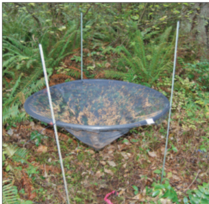
Figure 1. Each seedtrap contained a circular frame, 1.0 m 2 (10.8 ft 2 ) in area, constructed of flexible plastic tubing. A semicircle of fiberglass screen was stapled to the frame to create a conical trap for collecting Douglas-fir seeds, cones, and other forest litter. The trap was suspended on rods approximately 0.75 m (2.5 ft) above the ground. (Photo by Timothy B. Harrington, 2008)
