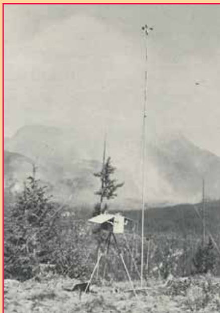
Portable fire weather station developed by the Forest Service's Intermountain Forest and Range Experiment Station of Forest Fire Research in use at the scene of the Coal Creek Fire.
