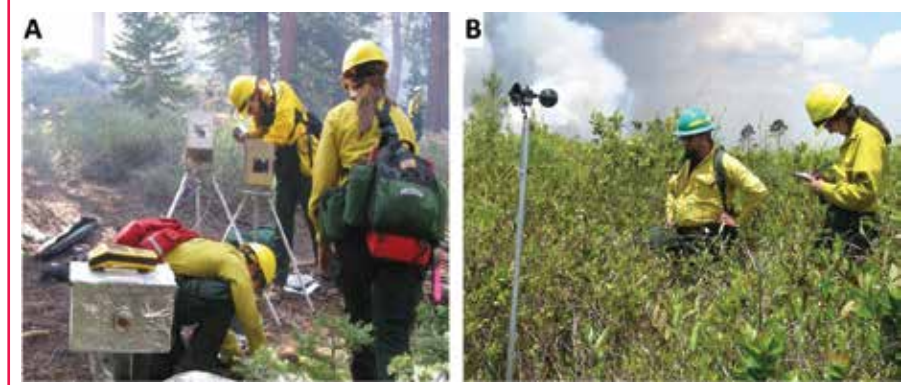
(A) Members of the Fire Behavior Assessment Team setting up the fire-resistant video cameras and radiant heat flux sensor on the Crag Fire in 2005 (photo: Rosalind Wu, Forest Service) and (B) gathering fuels data near the anemometer on the Georgia Bay Complex in 2007 (photo courtesy of Adaptive Management Services Enterprise Team).
