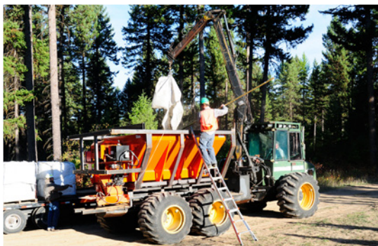
Use of bulk bags to improve transport and filling efficiency.
