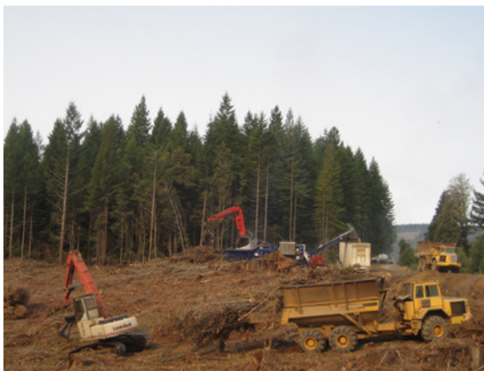
A centralized biomass recovery operation using modified dump trucks and all-wheel-drive chip trucks.
