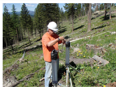
A hydrologist measuring hydraulic conductivity on a biomass utilization site.
