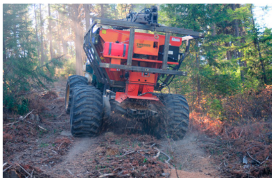
Applying material on a log skid trail with prototype biochar spreader.
