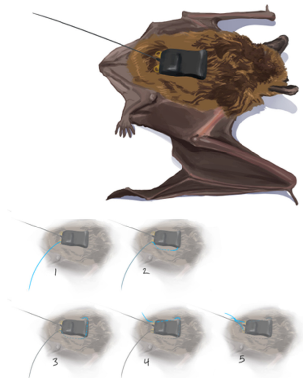
Figure 3. Diagram of suture placement to affix GPS tag to a big brown bat ( Eptesicus fuscus ). (1) Suture with needle is passed downwards through the loop at the back right of the tag and is put through the skin into the subcutaneous (SQ) space; (2) needle (& suture) is tunneled cranially in the SQ space and pulled out at the cranial aspect of the tag and passed through the “tube” in the tag; (3) needle is pulled out the left side of the “tube” and inserted into the SQ space and tunneled caudally through the SQ space to the caudal aspect of the tag; (4) needle is pulled out of the SQ space and upwards through the loop at the back left of the tag; and (5) ends of the suture are tied together using several knots thrown over the site where the antenna leaves the tag.
