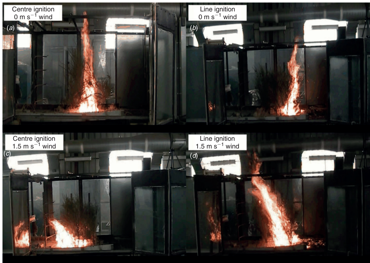
Fig. 5. Images of fire as viewed from the lateral camera in its flame spread direction. Those cases are for medium bulk density of (a) 3.17; (b) 4.00; (c) 3.80; and (d) 3.74 kg m -3 of the fuel bed. The imposed mean wind flow is from right to left.
