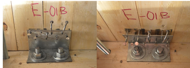
Figure 7: Connector failure Test 05
