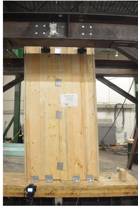
Figure 17: Test 23- (2) 0.61m walls with vertical joint
