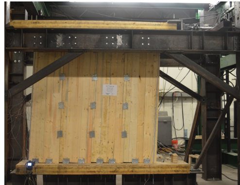
Figure 18: Test 26- (4) 0.61m walls with vertical joints
