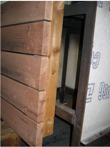
Figure 7. Vertically mounted redwood boarding with edges showing the pitch oozing out from radiant heating by the propane pool fire.
