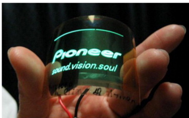
Figure 7 Flexible display on CNF substrate. (Reprinted with permission from [56]; Copyright 2009 Elsevier)
